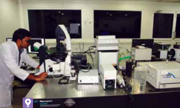
Laser Scanning Confocal Microscope for viewing structures inside cells by optical sectioning
