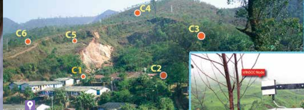
Munnar, Kerala: Amrita's detection system monitors soil conditions and sends an alert when landslides are imminent
