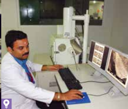
Raman Confocal Microscope for Raman imaging of cells and their internal structures
